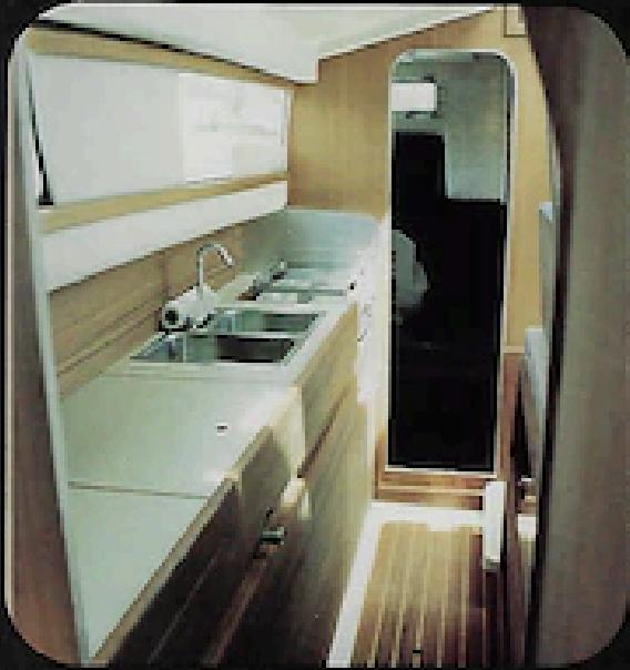
**GALLEY** — The galley is situated in the starboard hull well away from through traffic and with a panoramic view through the wide cabin windows. The galley comes complete with propane oven and broiler, a three-way fridge and pressurized hot and cold water to the sink. There is ample work surface, drawers and cupboard space.
