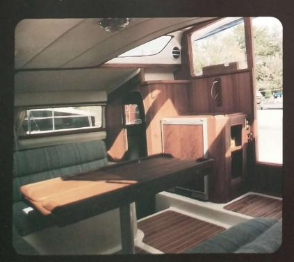
**VENTILATION** — The four large roof hatches and removable pilot house windows create a through-draft even on windless days because of convection currents.
