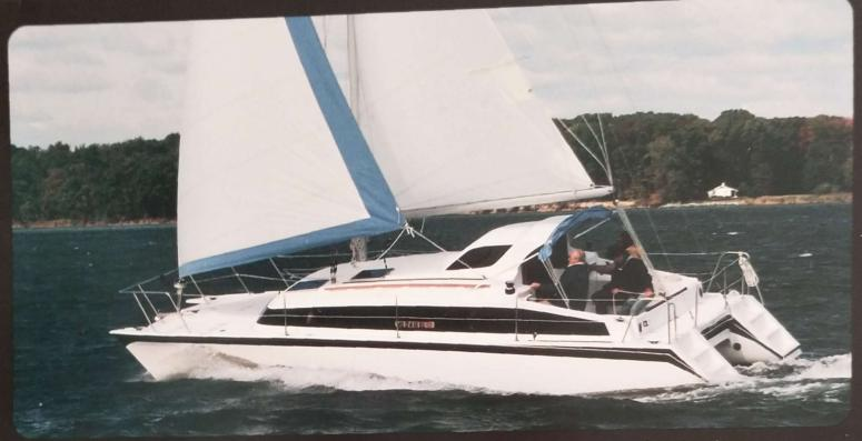
GEMINI 3400 with molded transom steps and adjustable underhung rudders. Either inboard or outboard engine.
